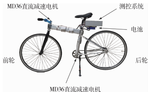
图 8 非同轴两轮平台物理样机 Fig. 8 Physical Prototype of Non-coaxial Two-Wheel Platform
